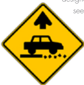
The current Pavement Ends sign can be difficult for older drivers with visual decline to read. (left)
